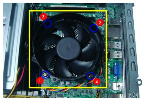
Note:CPU Fan has been highlighted with the yellow rectangle as above image shows.Please detach the CPU
